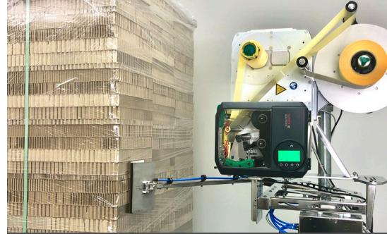
The label is printed with the XPA 936, the vacuum pad takes the label and the Rotor-Long applicator applies it accurately to the stationary/stopped pallet with a swing motion.
