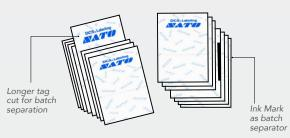
The printer separates tags by cutting the first tag longer or using the ink ribbon mechanism to place an ink mark on the side of each batch separator tag.
