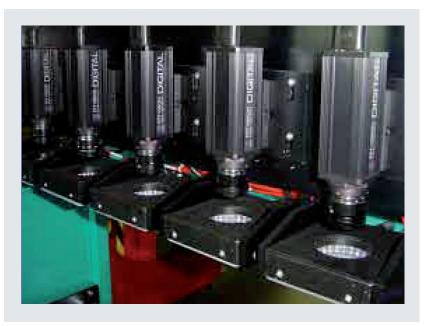
makes a final pass/fail decision based on certain criteria configured by the operators. Inspection results are also stored in a text file located on the vision PC for future reference (Production History).
